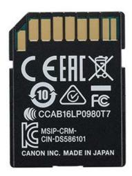
A rear view of the Wi-Fi Adapter W-E1. This accessory card will add wireless communication features to EOS 7D Mark II, EOS 5DS, and EOS 5DS R cameras, once a firmware upgrade has been installed in the host camera.
